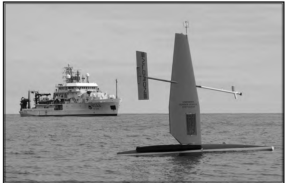
Saildrones have been used throughout the United States to map the seafloor. Last year was the first time the vessels traversed the Gulf of Maine. Saildrone photo.
