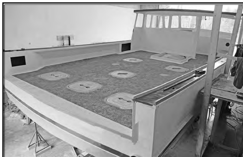
A lobster boat at Pat Feeney's shop with a SoftSand deck. SoftPoint Industries photo.
